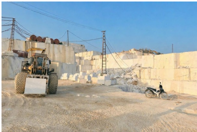
Active quarry face — block extraction
